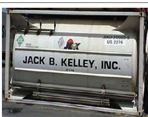
Specialized Intermodel Tank : Tank Within a Tank (Tangki Intermodel Khas : Tangki Dalam Tangki)
