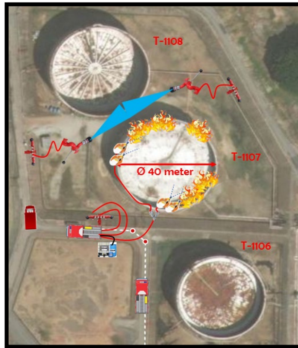
Gambar 5.3: Contoh susun atur pemadaman rim seal fire
